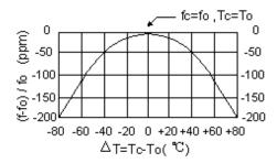
The curve shown above accounts for resonator contribution only and does not include oscillator temperature characteristics.
