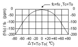
The curve shown above accounts for resonator contribution only and does not include LC component temperature characteristics.
