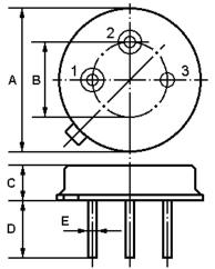
PinConfiguration1Input / Output2Output / Input3Case Ground
