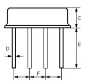
PinConfiguration1Input / Output4Output / Input2/3Case Ground
